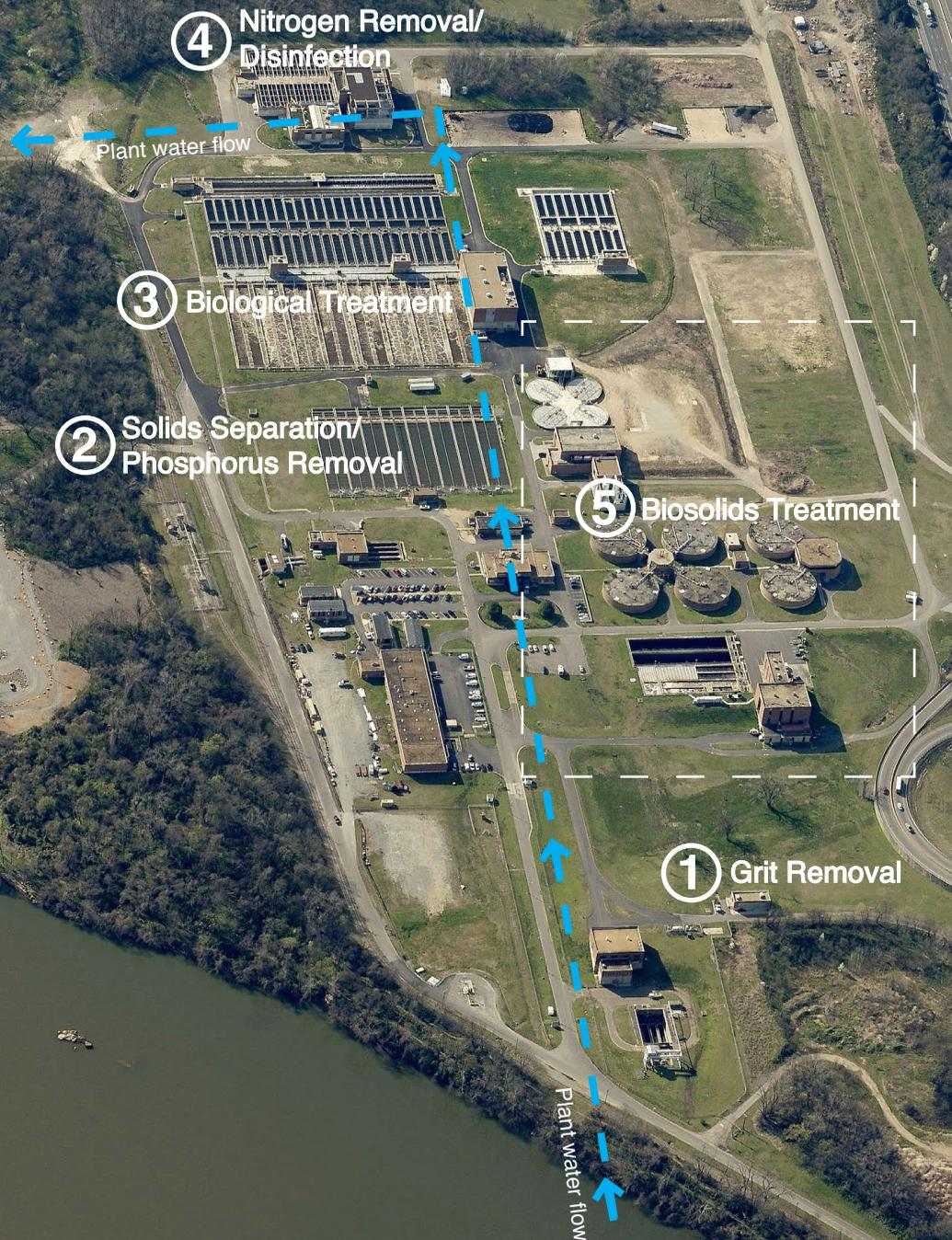
**1** In this preliminary treatment stage, wastewater flows to the headworks by gravity. Grit, rags, and heavy debris are removed and taken to a landfill off-site. Water is pumped from the lift station to the primary clarifiers.
