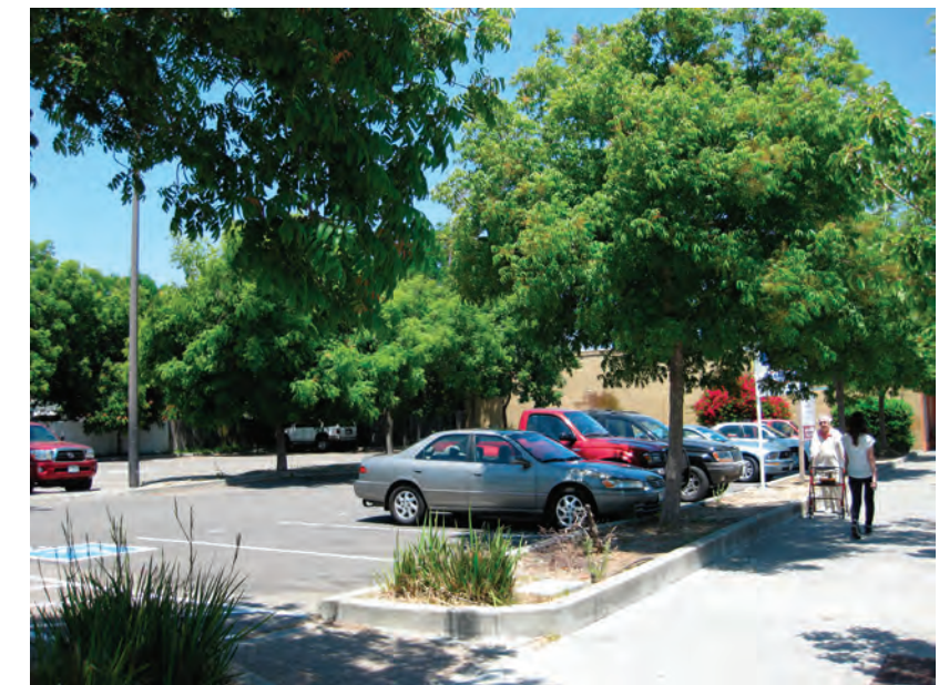
REAR PARKING LOT PRECEDENT Surface parking lots should be located in the rear or on the side of buildings. Minimum percentages of vegetation, plantings, and trees help to reduce heat islands, handle stormwater, and increase livability
