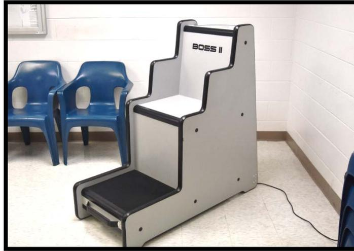
The **BOSS Chair** or **Body ORIFICE Security Scanner** is a non-intrusive scanning system designed to detect small metallic objects such as mobile telephones and weapons, concealed within abdominal cavities and the shin area. This chair is able to detect many items, from large knives to small gun components, which may be hidden by prisoners with the intention of smuggling them into establishments.
