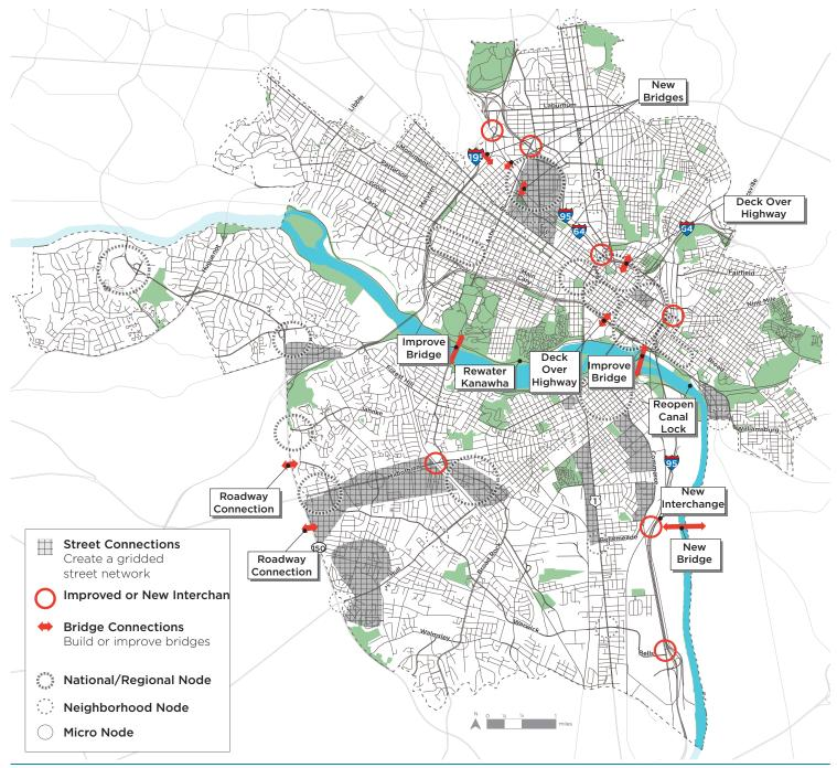
FIGURE 30 // Connections, Interchanges, and Bridges Map
