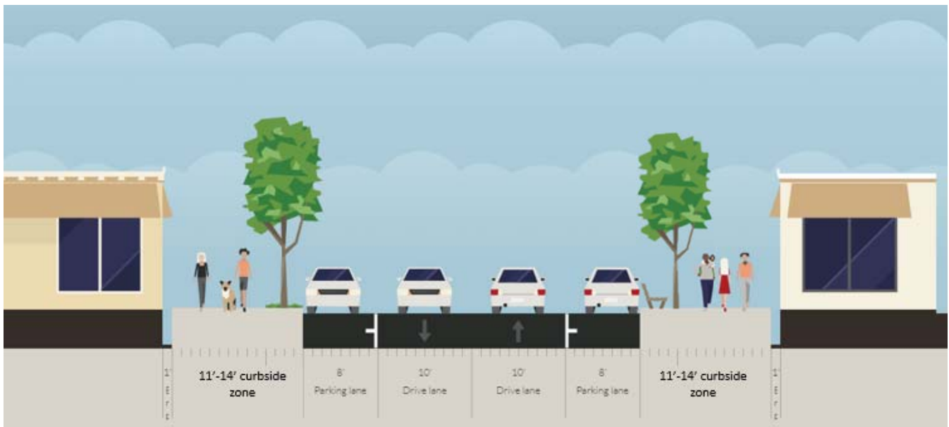
Figure 11 - Typical Base Cross Section
