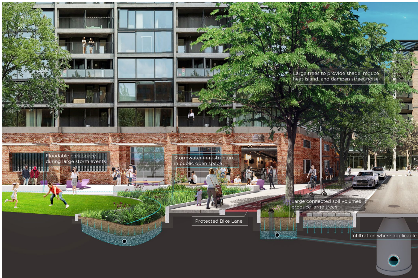
FIGURE 17 // Example illustration of Park Space that Can Also Hold Flood Water Volume
