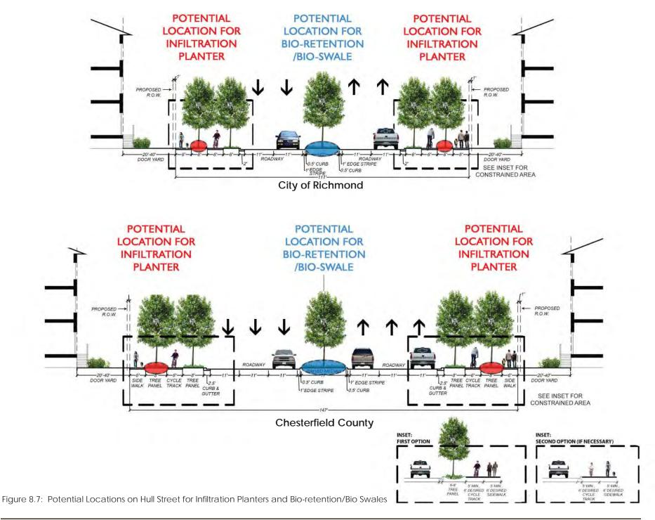
reaching natural watercourses<sup>1</sup>. Visually pleasing and cost-effective, bioswales enable the usage of narrow spaces, such as medians, for storm water mitigation.
